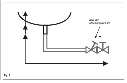
If the opening times were to be longer, the suction would be reduced and only the hot boiler water would be discharged, resulting in a waste of energy.
